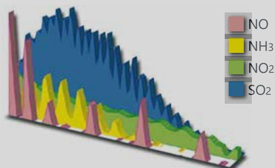
Several gases can be measured in a same analyser if the sample gas composition is compatible with the selected algorithms and wavelengths. The analyser gives high measurement selectivity thanks to the recognition of the specific UV absorption spectrum of gases by using proprietary algorithms.
